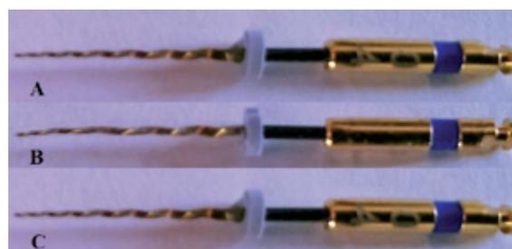
Fig. 2. Hyflex CM Files. A – before use. B – after use. C – after heat treatment
