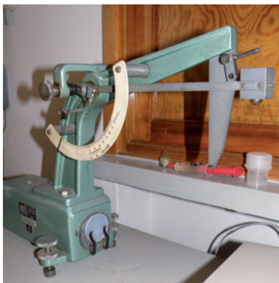
Fig 2. The pendulum used for testing shock elasticity using Schob's method
