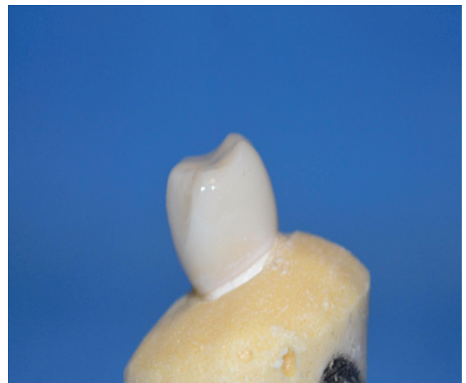
Fig. 3. Chipping of the veneering porcelain of a specimen in the ZVP (zirconia copings veneered by heat-pressing technique) group (cohesive failure)
