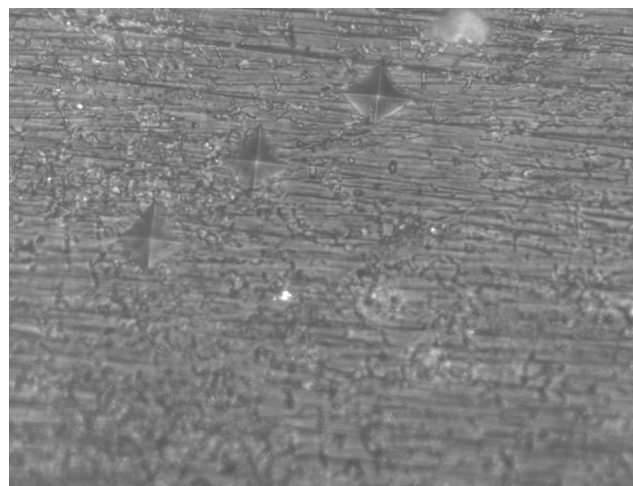
Fig. 1. Selected sample before demineralization (×10; Vickers microhardness tester). The sample shows uniformity
