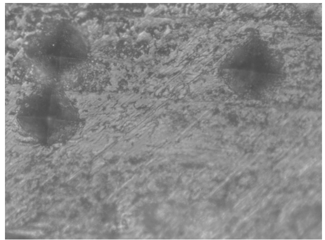
Fig. 5. Selected sample in the fluoride varnish group with 1% AgNP after treatment ( \times 40 ; Vickers microhardness tester). The sample exhibits less demineralization and porosity compared to the control group
